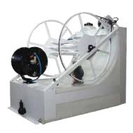
The Aqua Reel Water Tank has a rotational molded polyethylene tank. It has a 125 gallon capacity and has a 250' live solution reel and 250' electric vacuum reel. This space saving design is 35" wide with auto fill and a powder coated frame.
